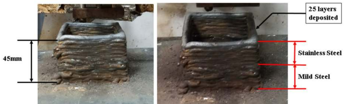
Figure 12. Mild steel and stainless steel bimetallic deposition.
