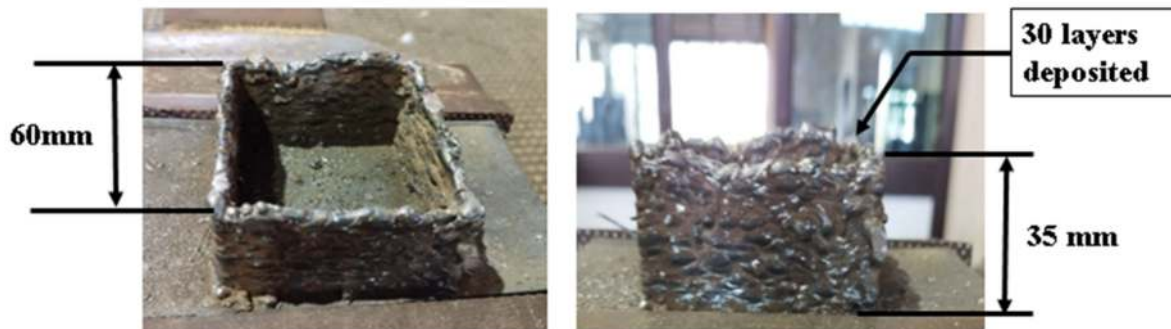
Figure 5. Mild steel sample deposited with CO 2 shielding gas.
