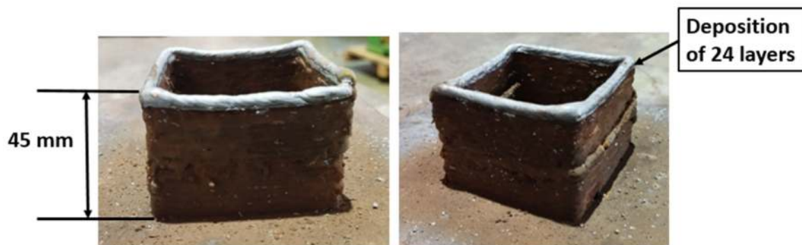
Figure 6. Mild steel sample deposited with argon shielding gas.
