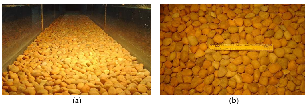
Figure 2. Photograph of an SGB in a laboratory flume (a); and a close view (b).
