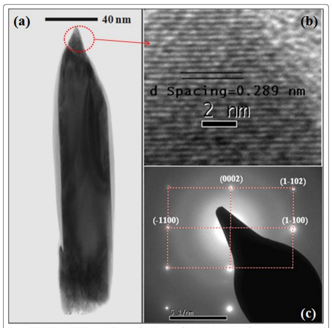
Figure 3 TEM, HRTEM, and SAED images.(a) TEM image, (b) HRTEM image of an InN NR taken on the tip of nanorod and (c) SAED pattern of an InN NR.
