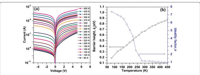
**Figure 7 Current versus voltage plots and variation of barrier heights and ideality factor**. (a) Current versus voltage plots of the InN NRs/ *n*-Si diode at different temperatures. (b) Variation of barrier heights and ideality factor with temperature.
