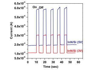
**Figure 8 A logarithmic plot of the transient photocurrent of InN NRs/n-Si heterojunction**. Measured at 3 and 5 V bias conditions.
