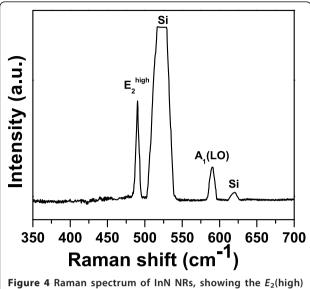
Figure 4 Raman spectrum of InN NRs, showing the  $E_2$ (high) and  $A_1$ (LO) phonon modes.
