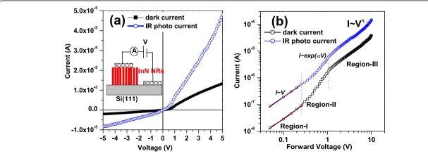
**Figure 5 Dark and IR photocurrent versus voltage plots, and log-log plots of the current-voltage**. (a) Dark and IR photocurrent versus voltage plots of the InN NRs/n-Si heterojunction diode. The inset shows the schematic diagram of diode. (b) Log-log plots of the current-voltage under forward bias of InN NRs/n-Si heterojunction measured at room temperature. The *I-V* plot is divided into three different regions.
