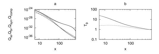
**Fig. 2** Variation of (a) dimensionless energy of Coulomb coupling (solid line), bremsstrahlung (dotted line), synchrotron (dash-dotted line), inverse Comptonization due to synchrotron photon (dashed line) processes in logarithmic scale, (b) corresponding ion (solid) and electron (dotted) temperatures in units of  $10^9$ K, as functions of radial coordinate for  $\dot{M} = 10$ . Other parameters are  $\alpha = 0.01$ , M = 10,  $\gamma = 1.345$ ; see Table 1 for details.
