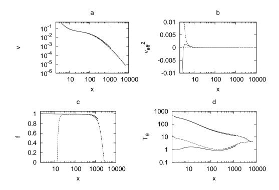
Fig. 7 Comparison between solutions for high and low  $\alpha$ : Variation of dimensionless (a) velocity, (b) square of convective frequency, (c) cooling factor, (d) ion (upper set of lines) and electron (lower set of lines) temperatures, a functions of radial coordinate, when solid lines correspond to  $\alpha = 0.01$  and dashed lines correspond to  $\alpha = 0.0001$ . Other parameters are  $\dot{M} = 0.01$ ,  $M = 10^7$ ,  $\gamma = 1.5$ , a = 0.
