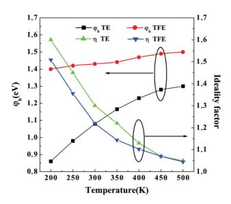
FIG. 7. (Color online) The temperature dependence of SBH and ideality factor obtained from TE and TFE models.
