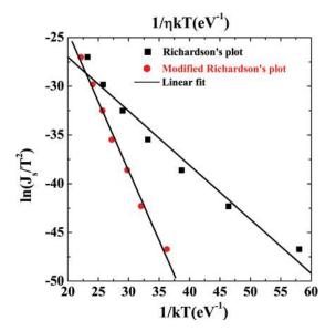
FIG. 4. (Color online) The conventional Richardson's plot of  $\ln(J_s/T^2)$  versus l/kT and the modified Richardson's plot of  $\ln(J_s/T^2)$  vs l/nkT.
