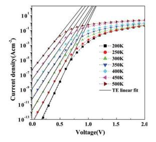
FIG. 3. (Color online) The forward J-V characteristics as a function temperature for the InN/GaN Schottky diode and the TE fitting to the J-V characteristics.
