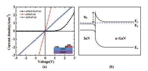
FIG. 2. (Color online) (a) Room temperature J-V measurement of the device. Inset shows the schematic of the device structure. (b) The equivalent schematic band diagram of the InN/GaN heterostructures.
