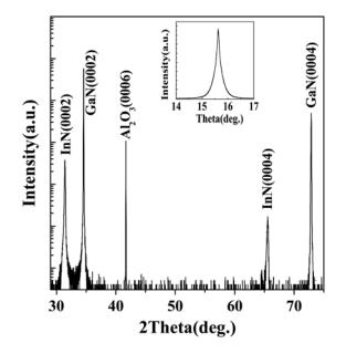
FIG. 1.  $2\theta$ - $\omega$  HRXRD scanning curve of InN film grown on GaN/sapphire template. Inset shows the XRC of the (0002) InN reflection.
