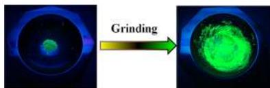
**Figure 3.** Photographic images of pristine and ground samples under a UV lamp.
