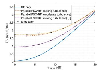
**Fig. 6.** The ASC v.s.  $\overline{\gamma}_{RF,D}$  for the parallel FSO/RF setup under varying optical link conditions ( $\mu_2 = 10$  dB, c = 6.7,  $\overline{\gamma}_{RF,E} = 5$  dB,  $m_D = 3$ ,  $m_E = 2$ ).
