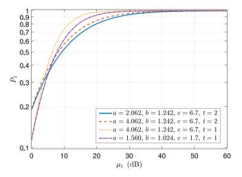
**Fig. 11.** The probability  $P_1$  versus  $\mu_t$  under varying FSO turbulence and FSO detection techniques ( $\overline{\gamma}_{RF,D} = 5 \text{ dB}, \overline{\gamma}_{RF,E} = 5 \text{ dB}, m_D = 3.2, m_E = 2$ ).
