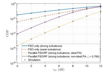
**Fig. 4.** The COP v.s.  $\gamma_{th}$  under the impact of FSO link turbulence and PA hardware efficiency ( $\mu_1 = 15$  dB, c = 6.7,  $P_{RF}^{cons} = 15$  dBm,  $m_D = 3.2$ ,  $\Omega_D = 1$ ).
