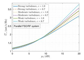
**Fig. 7.** The ASC versus  $\mu_2$  under varying FSO link conditions and FSO receiver pointing errors ( $\overline{\gamma}_{RF,D} = 10$  dB,  $\overline{\gamma}_{RF,E} = 5$  dB,  $m_D = 3$ ,  $m_E = 2$ ).
