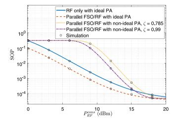
**Fig. 8.** The SOP versus  $P_{RF}^{cons}$  under the impact of PAs with different levels of hardware efficiency (weak FSO turbulence,  $\mu_2 = 5$  dB, c = 6.7,  $m_D = 3$ ,  $m_E = 2$ ,  $\Omega_D = 1$ ,  $\Omega_E = 0.01$ ).
