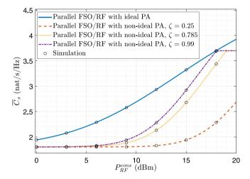
**Fig. 5.** The ASC v.s.  $P_{RF}^{cons}$  under the impact of PAs with varying levels of hardware efficiency (strong FSO turbulence,  $\mu_2 = 5$  dB, c = 1.0,  $m_D = 3$ ,  $m_E = 2$ ,  $\Omega_D = 1$ ,  $\Omega_E = 0.01$ ).
