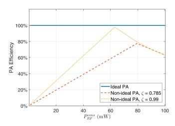
Fig. 2. PA efficiency v.s. P<sub>RF</sub><sup>cons</sup> for PAs with varying levels of PA efficiency.
