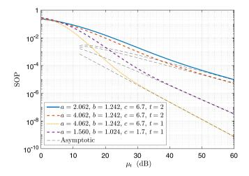
**Fig. 10.** The SOP versus  $\mu_t$  for various FSO turbulence scenarios and FSO detection techniques ( $\overline{\gamma}_{RF,D} = 5 \text{ dB}$ ,  $\overline{\gamma}_{RF,E} = 5 \text{ dB}$ ,  $m_D = 3.2$ ,  $m_E = 2$ ).
