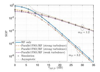
**Fig. 9.** The SOP versus  $\bar{\gamma}_{RF,D}$  for the parallel FSO/RF setup under varying optical link conditions ( $\bar{\gamma}_{RF,E} = 0$  dB,  $m_E = 2$ , c = 6.7, and  $\mu_2 = 10$  dB).
