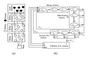
Fig. 1: a) Network scenario b) Relay node state model
