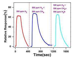
**Figure 8.** Cross selectivity response curve for various gases mixture (500 ppm H<sub>2</sub>, 500 ppm H<sub>2</sub> + 500 ppm CH<sub>4</sub> and 500 ppm H<sub>2</sub> + 500 ppm CH<sub>4</sub> + 500 ppm H<sub>2</sub>S) at 150 °C operating temperature.
