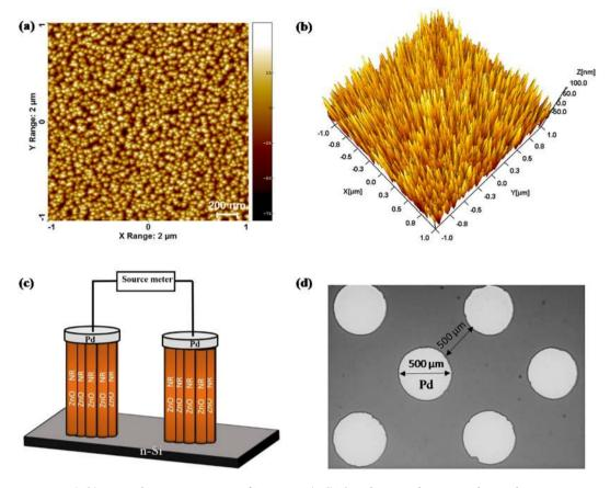
**Figure 1.** (**a**,**b**) 2-D and 3-D AFM images of ZnO NRs; (**c**,**d**) The schematic diagram and optical microscope image of the device.
