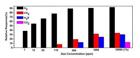
Figure 7. The selectivity histogram of the sensor to H<sub>2</sub>, CH<sub>4</sub>, H<sub>2</sub>S and CO<sub>2</sub> at 175 °C operating temperature.
