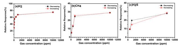
**Figure 4.** (a-c) Hysteresis studies for  $H_2$ ,  $CH_4$  and  $H_2S$  at 150 °C for increasing and decreasing gases concentration.
