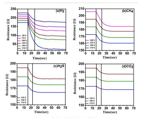
**Figure 5.** Resistance verses time curve for (**a**)  $H_{2}$ , (**b**)  $CH_4$ , (**c**)  $H_2S$  and (**d**)  $CO_2$  gases with 1% concentration at various temperatures.
