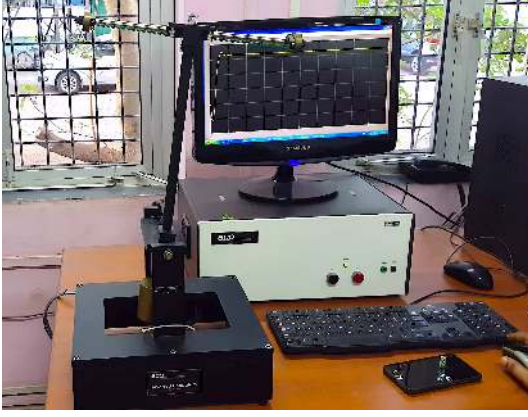
Fig. 2: Laboratory setup of pendulum system, ECP-Model 505.
