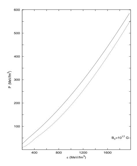
Fig. 2. Equation of state, pressure versus energy density, with a magnetic field having central value  $B_c = 10^{17}$  G (solid line) and without magnetic field (dashed curve).
