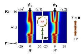
FIG. 6. WG2: Prototype waveguide isolator with 8.75% nonlinearity in the optical medium where one-way-traffic is active in the backward direction (from P2 to P1). Normalized backward propagations of (a.1)  $\psi_0$  and (a.2)  $\psi_1$  from P2 to P1 for anticlockwise dynamical EP-encirclement scheme where both of them are converted to  $\psi_0$  at P1. Here, for forward propagation,  $T \approx 0$ .
