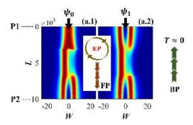
FIG. 5. WG1: Prototype waveguide isolator with 3.75% nonlinearity in the optical medium where one-way-traffic is active in the forward direction (from P1 to P2). Forward propagations of (a.1)  $\psi_0$  and (a.2)  $\psi_1$  from P1 to P2 for clockwise dynamical EP-encirclement scheme where both of them are converted to  $\psi_1$  at P2. For backward propagation,  $T \approx 0$ .
