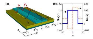
FIG. 1. (a) Schematic of the proposed specialty optical waveguide. x and z represent the transverse and propagation directions respectively. (b) Transverse profile of n(x): Blue solid line shows the Re(n), and the brown dotted line shows the Im(n) for the specific parameter set ( $\gamma = 0.008$ ,  $\tau = 3.161$ ) at EP.
