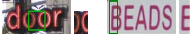
Figure 4 Typical challenges in character detection. (a) Inter-character confusion: A window containing parts of the two o 's is falsely detected as x . (b) Intra-character confusion: A window containing a part of the character B is recognized as E .
