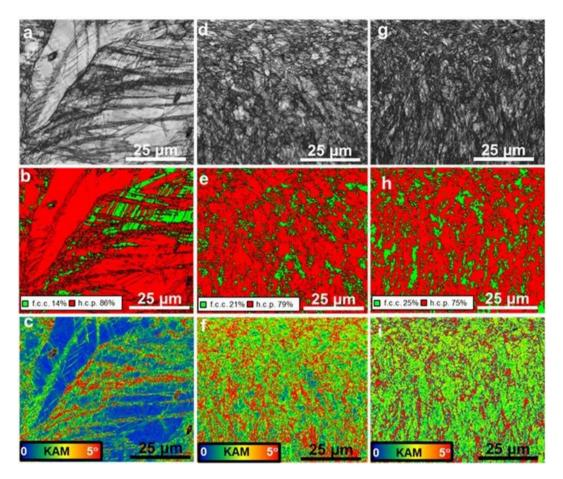
**Figure 3.** (a–c) EBSD image quality, phase, and KAM maps for the as-homogenized reference sample (d–f) image quality, phase, and KAM maps for the 350 RPM processed sample (g–i) image quality, phase, and KAM maps for the 650 RPM processed sample after room temperature tensile deformation at a strain rate of  $10^{-3}$  s<sup>-1</sup>. RPM: rotations per minute; KAM: kernel average misorientation.
