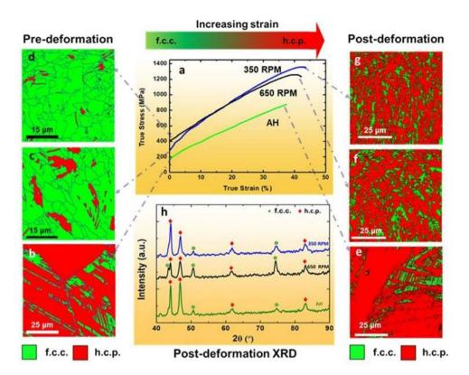
**Figure 2.** (a) True stress-true strain curves for the as-homogenized and FSP samples deformed at room temperature at an initial strain rate of  $10^{-3}$  s<sup>-1</sup>, (**b**-**d**) EBSD maps showing f.c.c.  $\gamma$ - and h.c.p. ε-phase fractions prior to tensile deformation and, (**e**-**h**) EBSD maps and corresponding XRD patterns showing f.c.c.  $\gamma$ - and h.c.p. ε-phase fractions after tensile deformation. AH: as-homogenized; RPM: rotations per minute.
