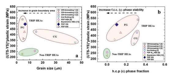
**Figure 4.** (a) Strength-ductility index (SDI) as a function of grain size and (b) variation of SDI as a function of  $\varepsilon$  phase fraction (prior to deformation) for grain-refined TRIP HEAs and non-TRIP HEAs. CG: coarse grained; FG: fine grained; FSP: friction stir processing; CR: cold rolling; RPM: rotations per minute.
