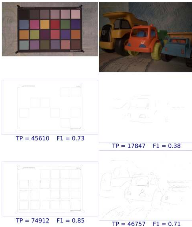
Figure 7. Results with pristine images with a particular threshold set. Top to bottom—Pristine Image, CED, Proposed edge detector ( high-resolution weblink )
