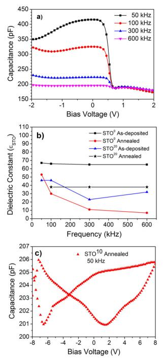
**Fig. 7.** (a) C-V characteristics of Ag/STO<sup>20</sup> (annealed)/p-Si MIS structure as a function of frequency, (b) STO thin film dielectric constants as a function of frequency, and (c) C-V hysteresis curve at 50 kHz for annealed STO<sup>10</sup> thin film.
