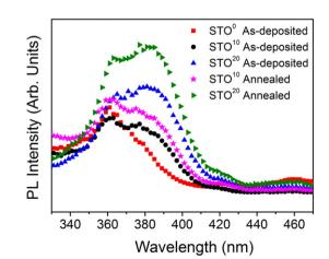
Fig. 6. Photoluminescence spectra of as-deposited and annealed thin films deposited on Si substrates.
