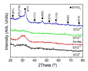
Fig. 1. GIXRD patterns of as-deposited STO<sup>20</sup>, annealed STO<sup>0</sup>, STO<sup>10</sup> and STO<sup>20</sup> thin films deposited on Si (100) substrates. Annealing was carried out at 700 °C for 1 h in  $O_2$  environment.
