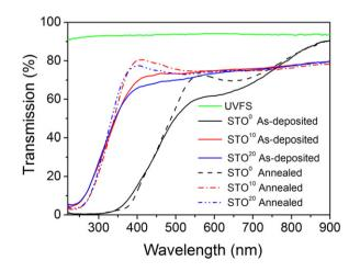
Fig. 3. Spectral optical transmission plots of as-deposited and annealed STO thin films deposited on UVFS substrates. Annealing was carried out at 700  $^\circ$ C for 1 h in O<sub>2</sub> environment.
