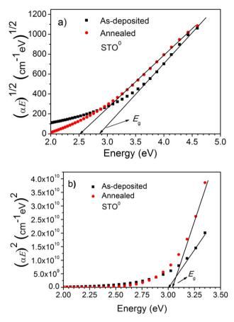
**Fig. 4.** Energy bang gap values of as-deposited and annealed STO<sup>0</sup> thin films corresponding to (a) indirect  $(\alpha E)^{1/2}$  vs. *E*, and (b) direct  $(\alpha E)^2$  vs. *E*.
