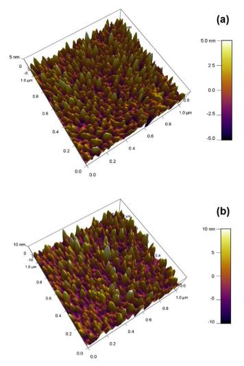
Fig. 2. 3D AFM surface morphologies of annealed STO thin films deposited using (a) 10%  $O_2$ , and (b) 20%  $O_2$  concentrations.
