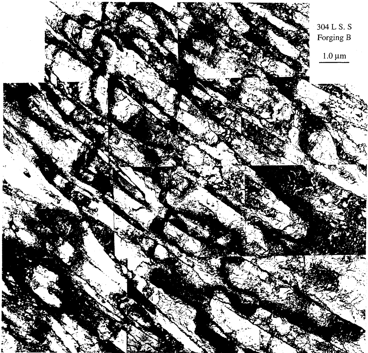
Fig. 15. Following a moderate deformation, \epsilon_{\text{VM}} \sim 0.2-0.3 , in a hammer forging of 304L S.S. (vendor B), a cell block structure of extended GNBs near the main slip plane is observed.
