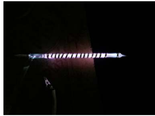
FIG. 3. Argon jet generated using the floating helix configuration.
