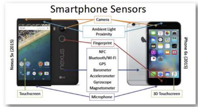
Fig. 14. Smartphones are equipped with a number of sensors. Data from these sensors can be combined in a judicious manner to perform multimodal user authentication. However, a number of research issues have to be resolved when designing such a solution. ©Debyan Deb.
