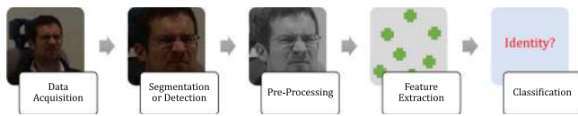
Fig. 1. General pipeline of a face recognition system. From a pattern recognition perspective, the most significant modules of a biometric system are the sensor module, the segmentation module; the feature extraction module; and the classification or decision-making module. Face image has been taken from the CMU Multi-PIE dataset [215].
