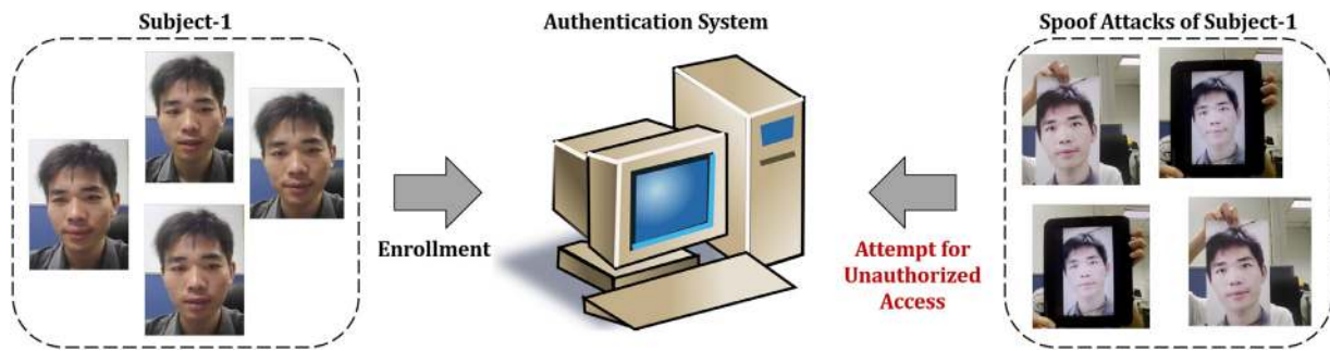
Fig. 12. Presentation attacks on a face recognition system where an adversary attempts to spoof the identity of Subject-1. Face images have been taken from the CASIA-FASD database [152].
