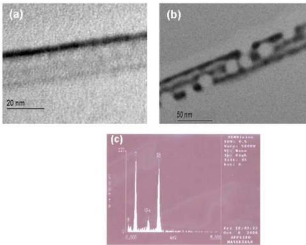
FIG. 2. (Color online) TEM images of layers (a) overoxidized at 1000 °C, (b) overoxidized at 925 °C showing SiO and SiGeO layers, and (c) EDS spectrum of SiGeO layer.
