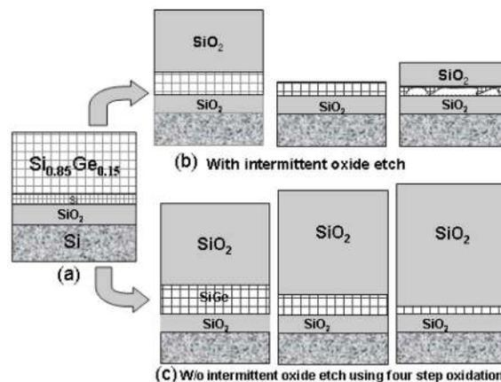
FIG. 1. (Color online) Schematic process flows of SGOI condensation with and without intermittent oxide etch: (a) As deposited, [(b) and (c)] flow with and without oxide etch, (d) overoxidized due to uncontrolled oxidation, and (e) high Ge content SGOI layer formed from controlled oxidation.
