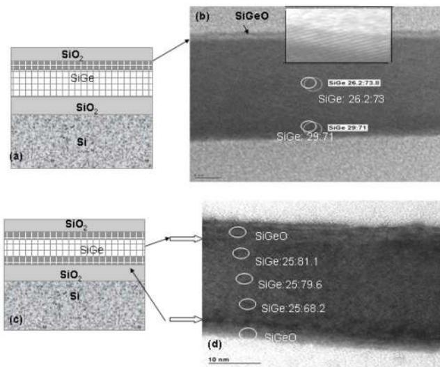
FIG. 3. (Color online) (a) Schematic of additional crystalline silicon germanium oxide (SiGeO) with SGOI. (b) TEM image of SGOI layer with additional layer at SiGe and top oxide. Inset shows the crystalline nature of the layer. (c) Schematic of double layers observed in SGOI layer. (d) TEM images showing the SiGeO oxide on both sides of the SiGe layer.
