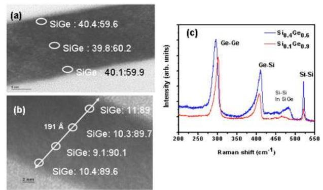
FIG. 4. (Color online) TEM images of (a) Si<sub>0.4</sub>Ge<sub>0.6</sub>OI layer and (b) Si<sub>0.10</sub>Ge<sub>0.90</sub>OI layer. (c) Raman data for the SGOI layers with 60% and 90% Ge.
