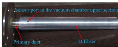
(a) Round secondary flow ejector geometry
