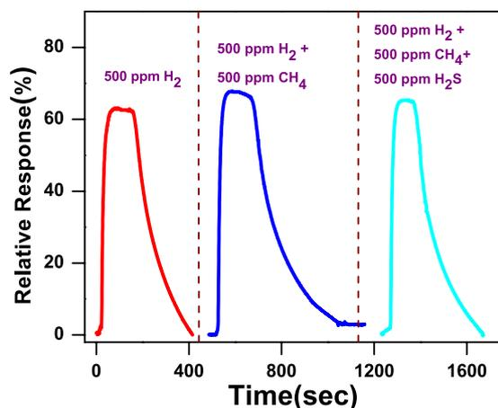
**Figure 8.** Cross selectivity response curve for various gases mixture (500 ppm H<sub>2</sub>, 500 ppm H<sub>2</sub> + 500 ppm CH<sub>4</sub> and 500 ppm H<sub>2</sub> + 500 ppm CH<sub>4</sub> + 500 ppm H<sub>2</sub>S) at 150 °C operating temperature.
