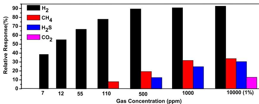
**Figure 7.** The selectivity histogram of the sensor to  $H_2$ ,  $CH_4$ ,  $H_2S$  and  $CO_2$  at  $175^\circ C$  operating temperature.
