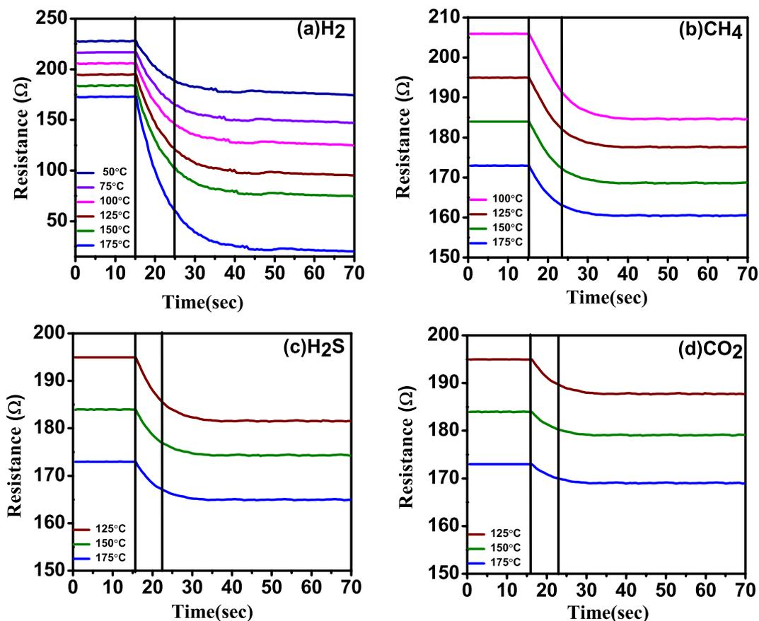
**Figure 5.** Resistance versus time curve for (a) H<sub>2</sub>, (b) CH<sub>4</sub>, (c) H<sub>2</sub>S and (d) CO<sub>2</sub> gases with 1% concentration at various temperatures.
