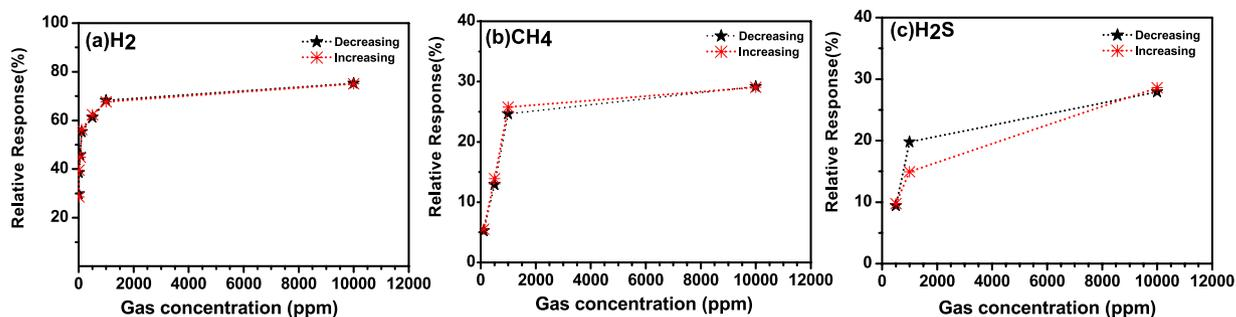
**Figure 4.** (a–c) Hysteresis studies for H<sub>2</sub>, CH<sub>4</sub> and H<sub>2</sub>S at 150 °C for increasing and decreasing gases concentration.
