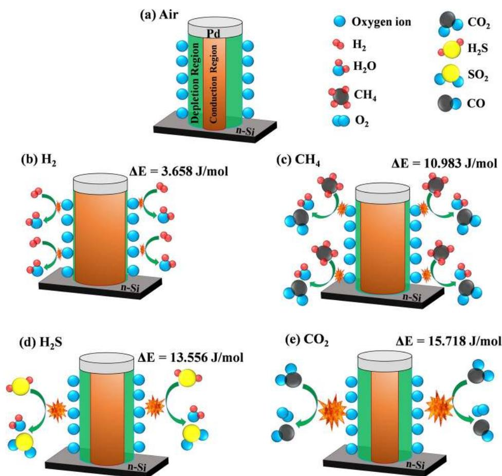
**Figure 9.** The gas sensing mechanism for sensor; a relative change in depletion region of ZnO NRs in presence of (a) Air, (b) H<sub>2</sub>, (c) CH<sub>4</sub>, (d) H<sub>2</sub>S and (e) CO<sub>2</sub> gases.
