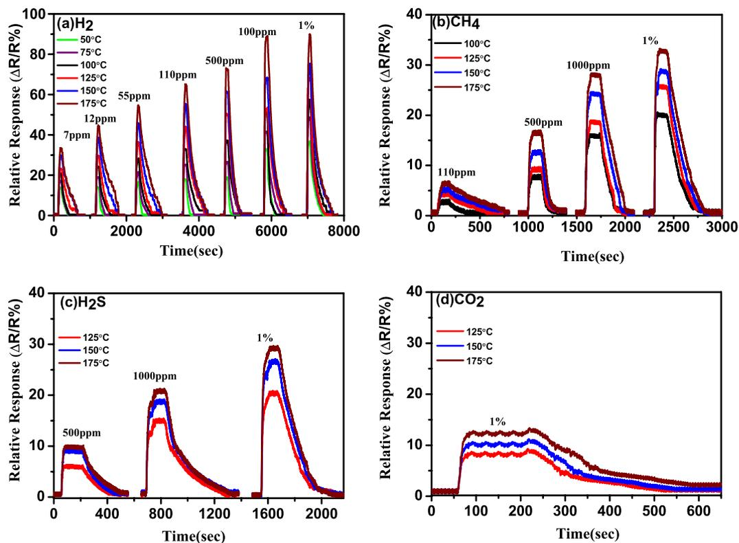
**Figure 2.** Sensor's relative response curve with time for 7 ppm to 10,000 ppm of gases: (a)  $H_2$ , (b)  $CH_4$ , (c)  $H_2S$  and (d)  $CO_2$ , at operating temperature ranging from 50 °C to 175 °C.
