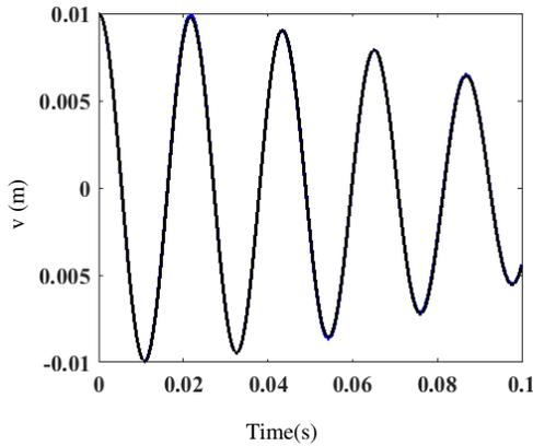
Fig. 18: Time history of shaft-disk system when subjected to spinning speed equal to 100 rad/s
