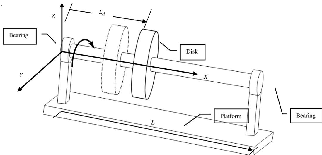
Figure 1: Rotor System with shaft and disk
