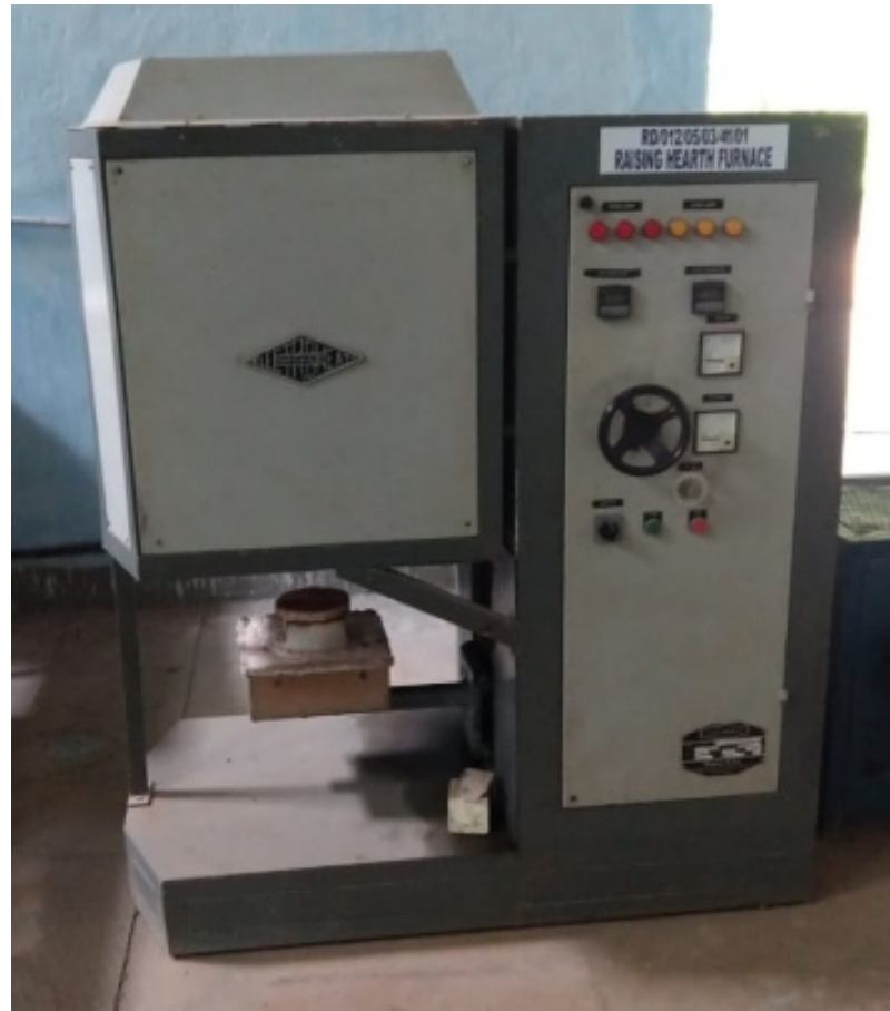
Figure 1. Raising Hearth Furnace (RHF).
