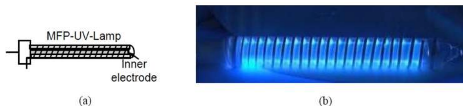
Figure 1. (a) Schematic view of MFP-UV-lamp and (b) Actual view of MFP-UV-lamp.
