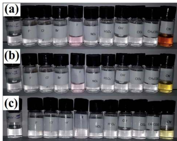
Fig. 1 Colorimetric analysis for (a) ionophore I, (b) ionophore II, and (c) ionophore III upon addition of different anions.
