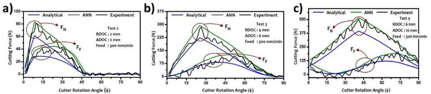
Fig. 5. Comparison of Measured and Predicted Forces: (a) Test No. 2; (b) Test No. 3; (c) Test No. 4
