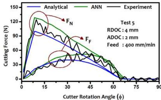
Fig. 6. Comparison of Measured and Predicted Forces (Test No.5)
