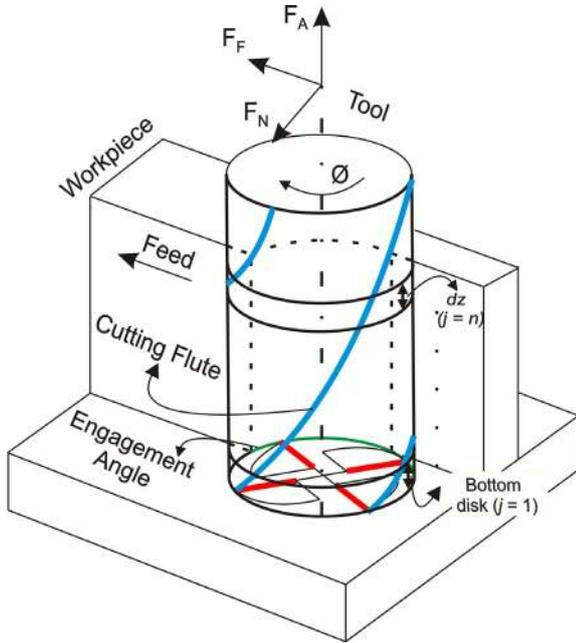
Fig. 1. Schematic of End Milling Process
