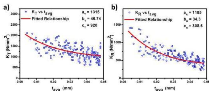
Fig. 3. Cutting Constant (Analytical Approach)
