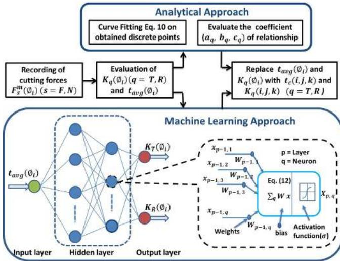
Fig. 2. Calibration of Cutting Constant
