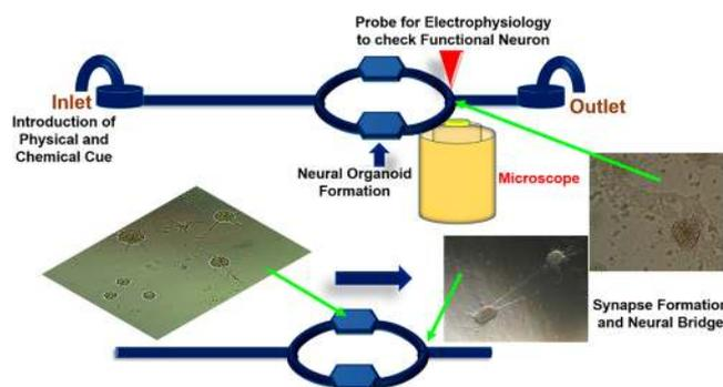
**Figure 1.** Cartoon represents design of 3D microfluidic platform for culture of neural organoid, real time monitoring of synapse formation and evaluation of functional neuron along with imaging.
