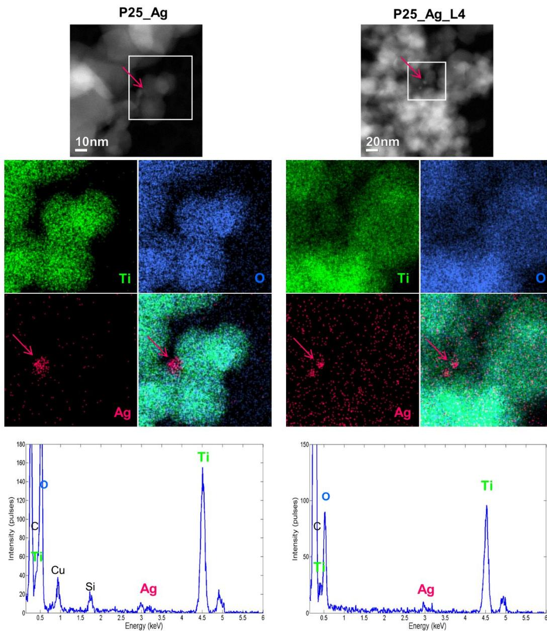
**Figure 7.** High angular annular dark field – STEM (HAADF-STEM) images (top) and EDX spectra (bottom) of P25\_Ag (left) and P25\_Ag\_L4 (right) samples. The elemental maps show the presence of the Ag nanoparticles on the surface of TiO<sub>2</sub>.
