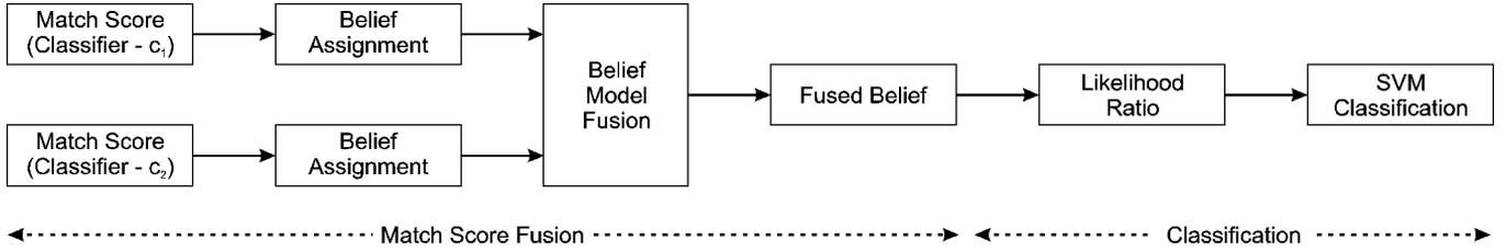
Fig. 1. Block diagram illustrating the steps involved in the proposed sequential match score fusion algorithm.
