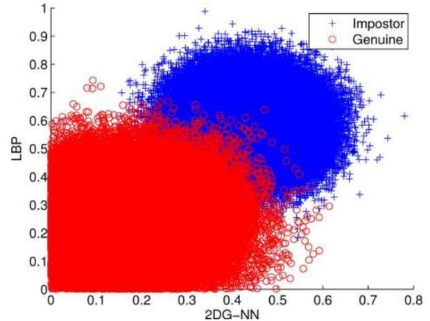
Fig. 7. Scatter plot shows that there is limited correlation between match scores obtained from LBP and 2DG-NN face recognition algorithms. Thus, score level fusion is expected to improve the matching performance.
