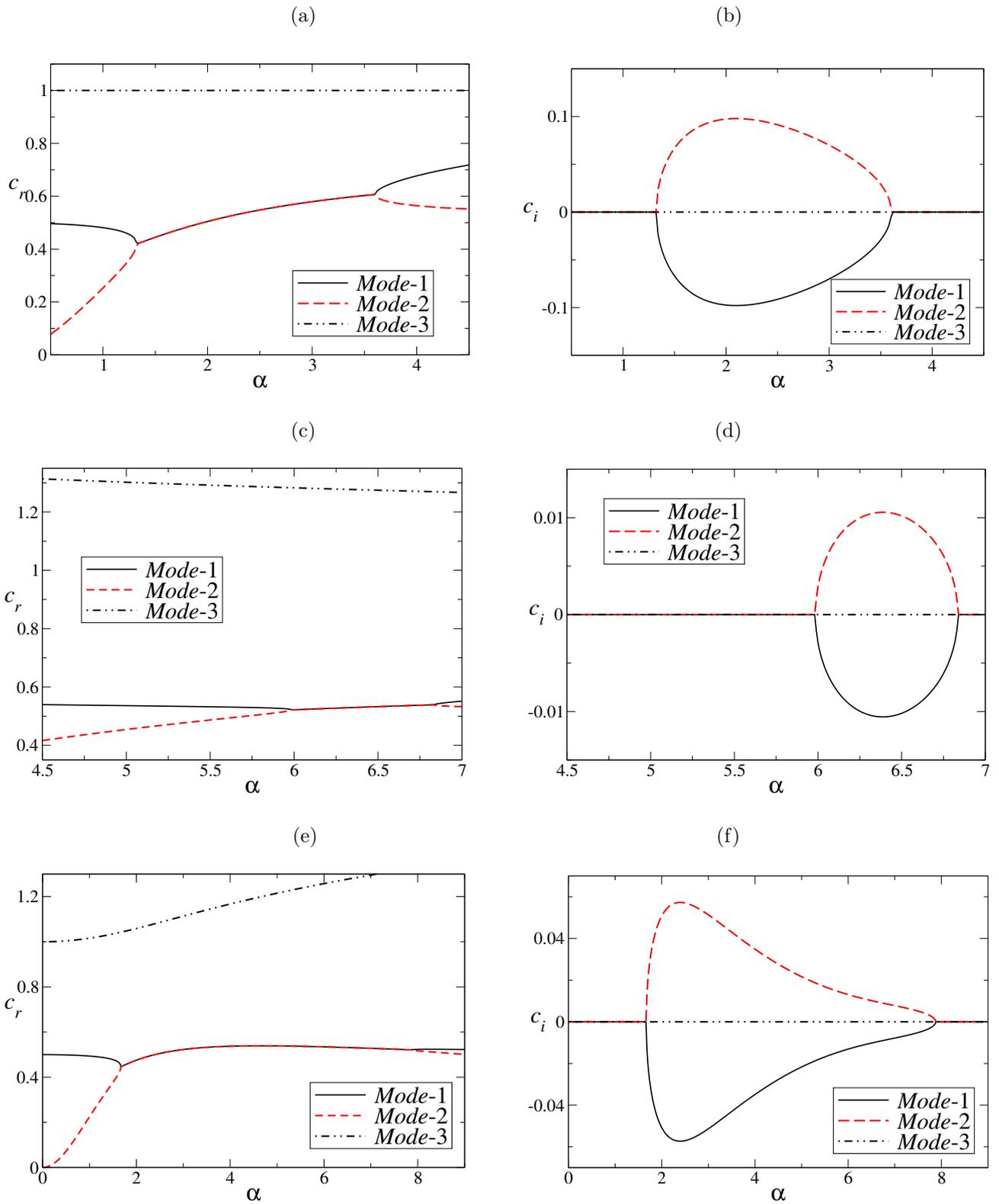
**Fig. 3** Real and imaginary parts of eigenmodes as a function of wave number  $\alpha$  when  $K_1 = 1, K_2 = 1.5, d = 0.4$  and  $G = 5/6$ : Fig. (a), (b) for  $\theta = 90^\circ, S = 0$ ; Fig. (c), (d) for  $\theta = 45^\circ, S = 0$ . Fig. (e), (f) are for surface tension parameter  $S = 0.02$  with  $\theta = 90^\circ$ . Here  $c_r$  and  $c_i$  represent real and imaginary parts of the eigenmodes.
