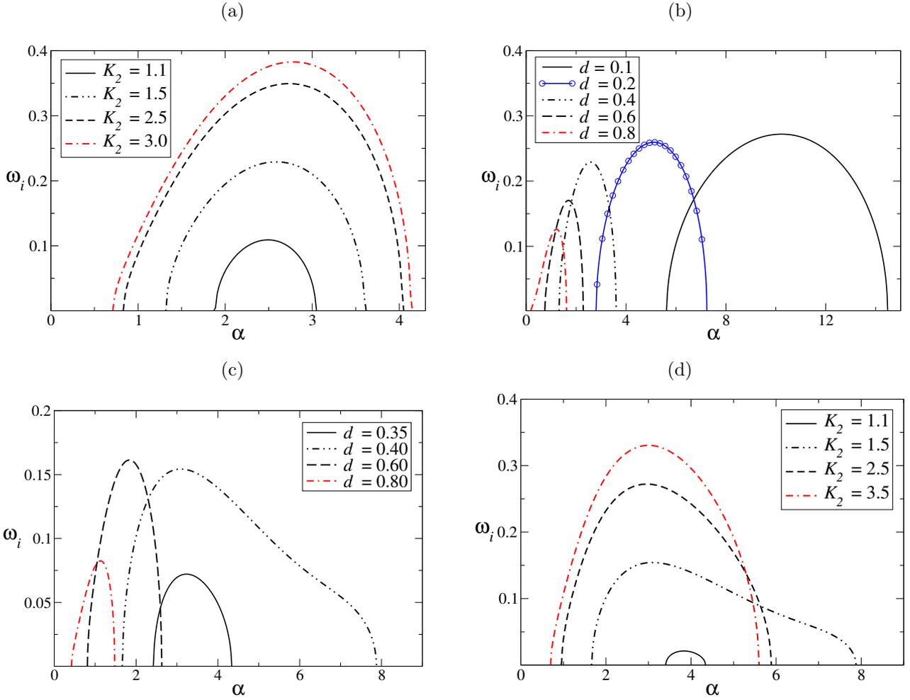
**Fig. 4** Influence of upper layer slope ( $K_2$ ) and effect of distance between the two interfaces ( $d$ ) on the growth rate  $\omega_i = \alpha c_i$  for  $K_1 = 1$ ,  $\theta = 90^\circ$ ,  $G = 1/Y$ . Fig. (a), (b) are without surface tension ( $S = 0$ ) and in Fig. (c), (d) surface tension  $S = 0.02$ . In Fig. (a), (c),  $d = 0$  and in Fig. (b), (d),  $K_2 = 1.5$ .
