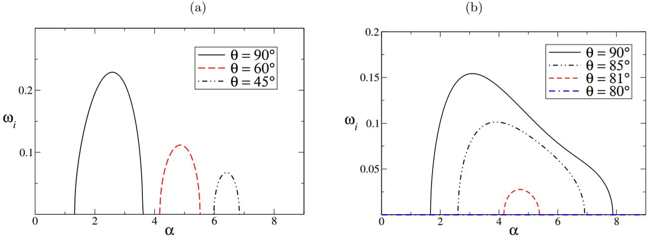
**Fig. 7** Influence of angle of inclination  $\theta$  on the growth rate  $\omega_i = \alpha c_i$  for  $K_1 = 1$ ,  $K_2 = 1.5$ ,  $d = 0.4$ :  $S = 0$  in Fig. (a) and  $S = 0.02$  in Fig. (b). The dimensionless gravity parameter,  $G = 5/6$ .
