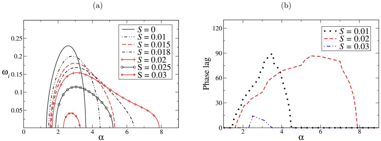
**Fig. 5** (a) Influence of surface tension on the growth rate ( $\omega_i$ ) and (b) Phase lag between the waves, at the free surface ( $h_2$ ) and the liquid-liquid interface ( $h_1$ ) for different surface tension parameter ( $S$ ) value. The other parameters are  $K_2 = 1.5$ ,  $d = 0.4$ ,  $\theta = 90^\circ$ ,  $G = 5/6$ .
