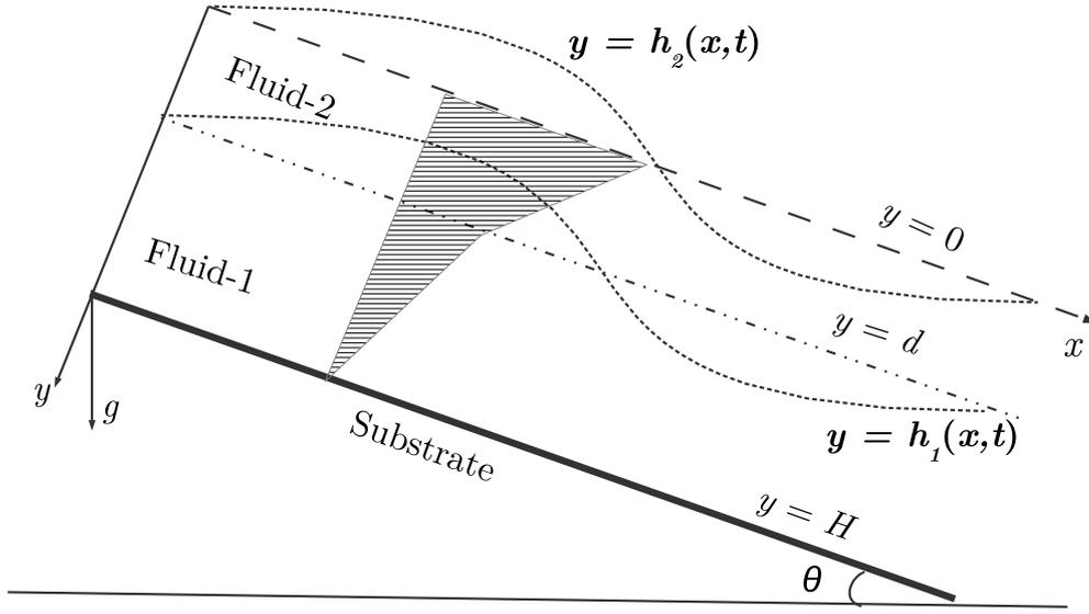
**Fig. 1** Schematic of the geometry for the flow system considered. Fluids ‘1’ and ‘2’ occupy the regions near the inclined plane ( $y = H$ ) and near the free surface ( $y = h_2(x, t)$ ) respectively.  $y = h_1(x, t)$  represents the liquid-liquid interface and  $\theta$  is the angle of inclination.
