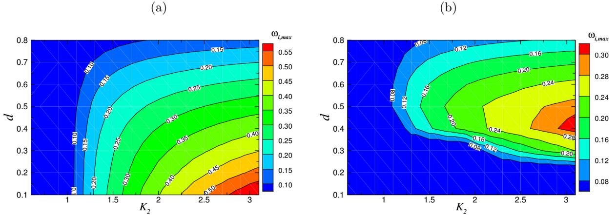
**Fig. 6** Contour plot of maximum growth rate  $\omega_{i,max}$  in  $K_2 - d$  plane: (a) in the absence of surface tension ( $S = 0$ ); (b) for surface tension parameter  $S = 0.02$ . The other parameters are  $K_1 = 1$ ,  $\theta = 90^\circ$ ,  $G = 1/Y$ .
