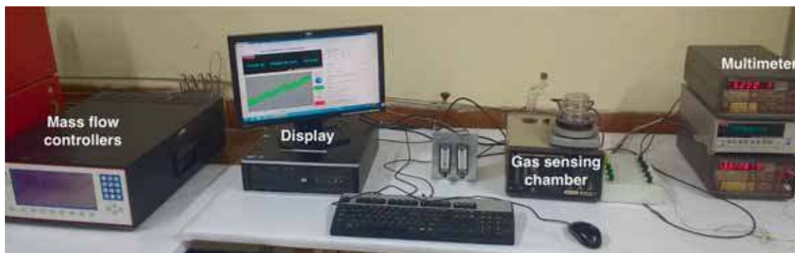
Figure 1. Gas-sensing setup for detection of acetone gas.
