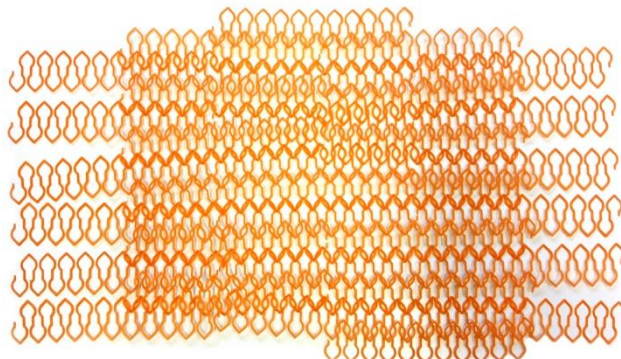
Figure 17: Variation to knit geometry and ability to stagger assembly using a running bond pattern. 3D printed on a Duplicator i3 (Wanhao, China) in ABS material.
