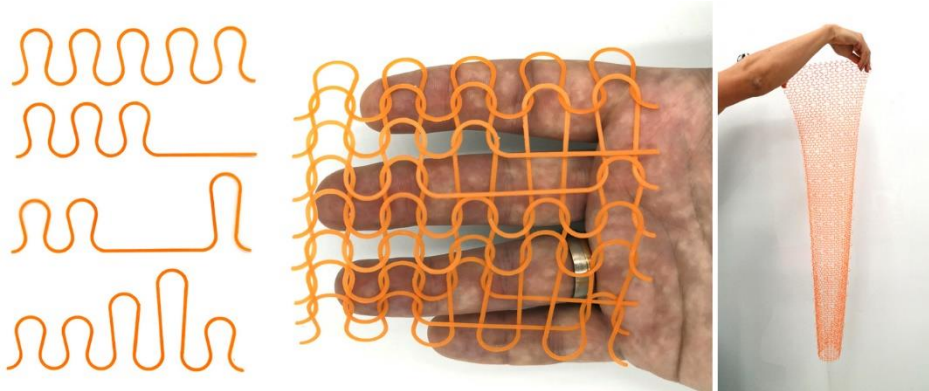
Figure 16: 3D printed sample of knit using desktop Wanhao Duplicator i3 (FDM) and ABS material on the left, with a 900mm sample printed on a BigRep ONE and PLA material on the right.
