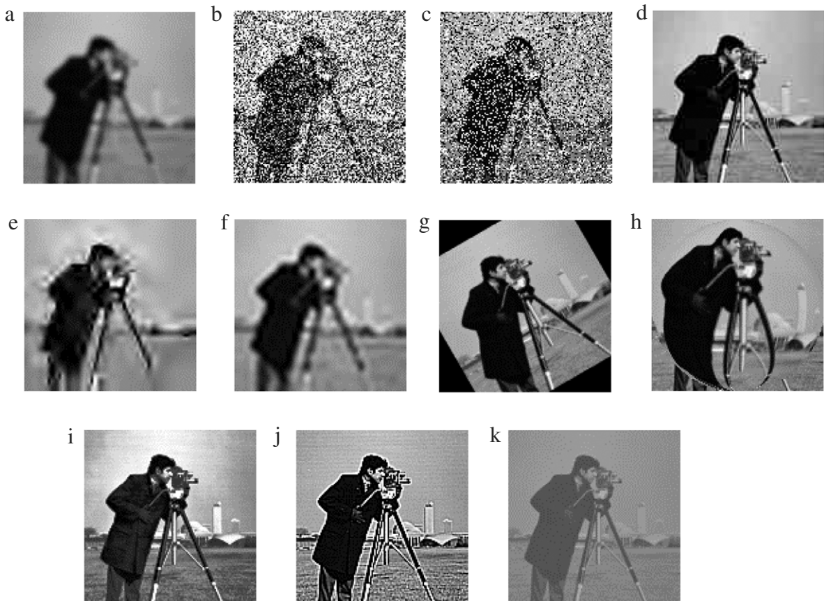
Fig. 7. Watermarked images after (a) Gaussian blurring ( 7 \times 7 ) (b) Gaussian noise addition (50%) (c) Salt & pepper noise addition (50%) (d) JPEG compression (80:1) (e) SPIHT compression (0.1 bpp) (f) Resizing ( 256 \rightarrow 64 \rightarrow 256 ) (g) Rotation ( 30^\circ ) (h) Wrapping (i) Histogram equalization (j) Sharpen (increased by 80%) (k) Contrast adjustment (decreased by 80%).
